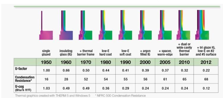
AAMA 1503-09, Voluntary Test Method for Thermal Transmittance and Condensation Resistance of Windows, Doors and Glazed Wall Sections is commonly used and widely accepted in the commercial industry for determining a product's condensation resistance factor (CRF). A CRF tool is also available on the AAMA website.
